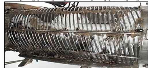
Non-uniform gaps, original grader Uniform gaps, modified grader
